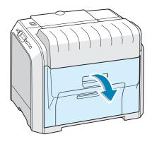
**2** Carefully remove the misfed paper in the direction, as shown. Go to step 6.
